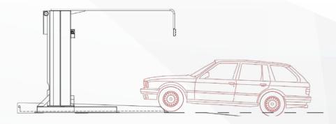
The shown above maximum angles have not to be exceeded. Wrong approach angles will cause serious manoeuvring & positioning problems on the parking system for which the local agency of Sanpark will not accepts responsibility.
