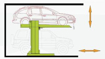
Before lowering the upper platform, the vehicle parked on the lower floor must be driven off!
