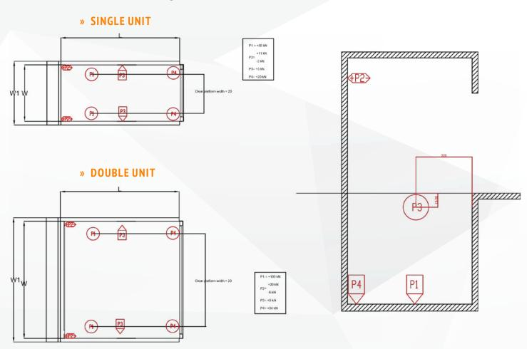
\* All static loadings include the weight of the car
