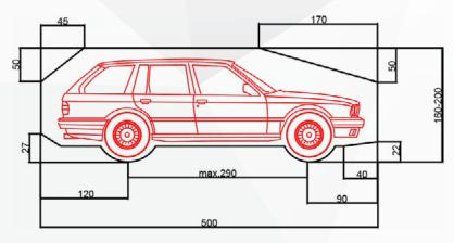
The total car height includes roof rail and antenna. Car height must not exceed the above max.car dimensions
